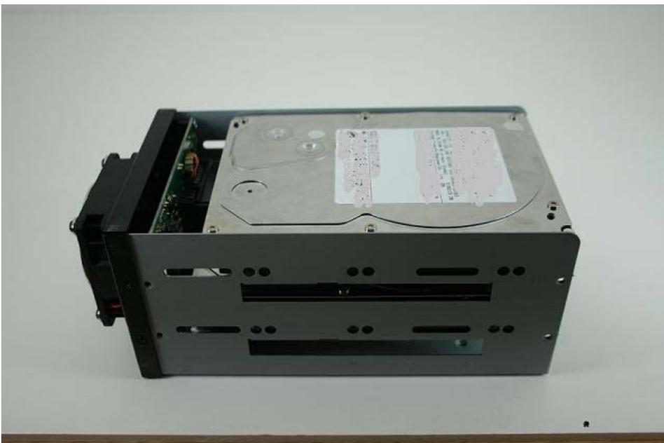
The screw holes of the drive will be aligned with the tray.
