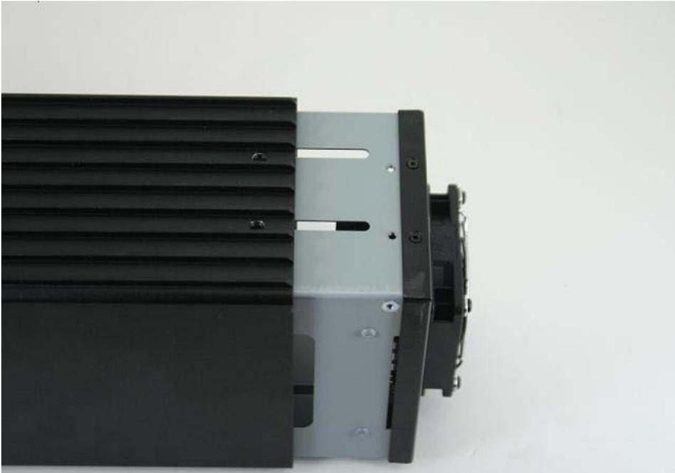
4. Remove 4 screws from the sides of the faceplate.
