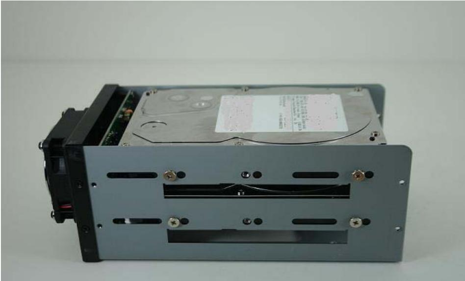
8. Place the faceplate on the front. Make sure you match the light indicators on the faceplate to the LED lights. Align the screw holes of the faceplate to the tray.
