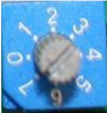
**Step 4.** Using a small, flathead screwdriver, turn the dial to the appropriate number of the setting you chose from Step 2. Once you have done this, lay the unit upright and set the unit where you would like it to be.
